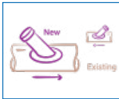
Direct to the public sewer via saddle connection
